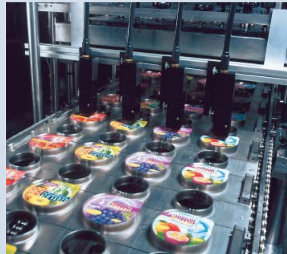
Synchronous individual marking with 4 alphaJET c4 printing heads in a multi-lane production plant
